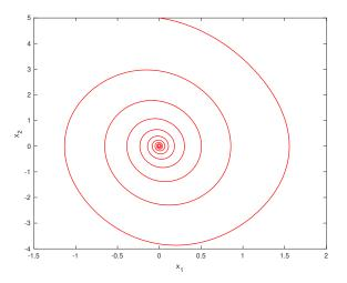
Solution of pendulum equation
